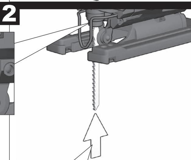
Press the saw blade into the Fixtec holder up to the stop.
