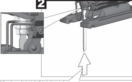
Press the saw blade into the Fixtec holder up to the stop. 将锯条完全压进Fixtec-装置。
